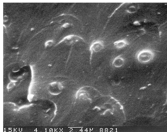
FIG. 4. SEM photomicrograph of the fracture surface of DGEBA/DDM/10% ECO. See Figures 1 and 3 for abbreviations.
